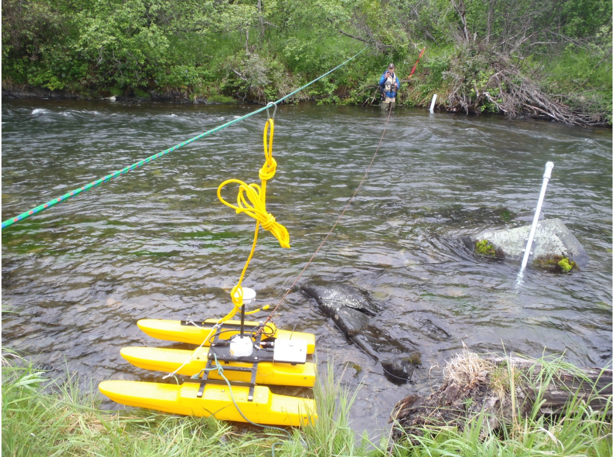
Figure 10. Manual Discharge Measurement at the Russian River Stream Gauge using the Sontek M9 River Surveyor ADCP
