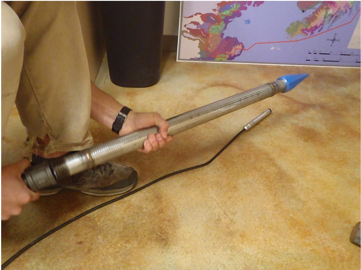
Figure 9. Ott Pressure Transducer and Well Casing
