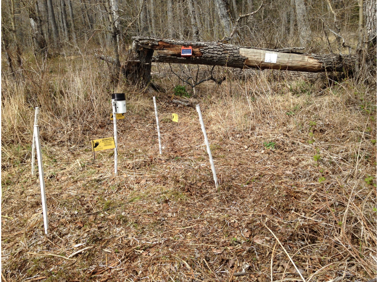
Figure 5. Upper Russian Lake Precipitation Gauge
